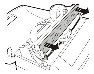
Figure 3-10 Removal of the ribbon cartridge
