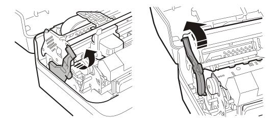
Figure 2-4 Lever for lifting the upper part of the mechanism
