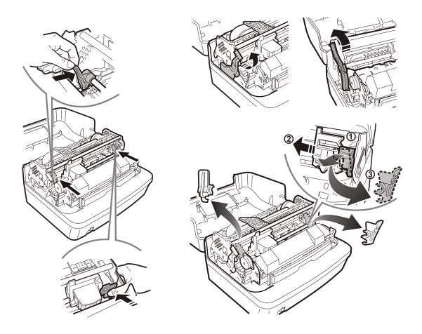
Figure 3-2 Removal of transport blocking devices
