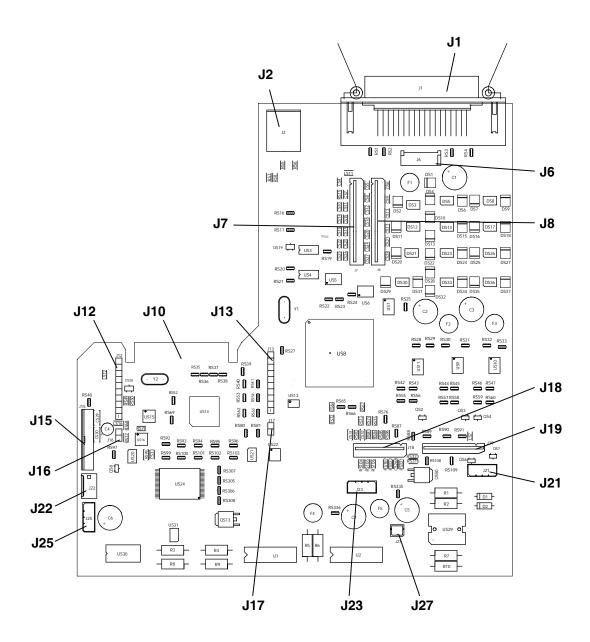
Figure 6-2 Motherboard PR2 plus (version with 1 RS232 serial interface)
