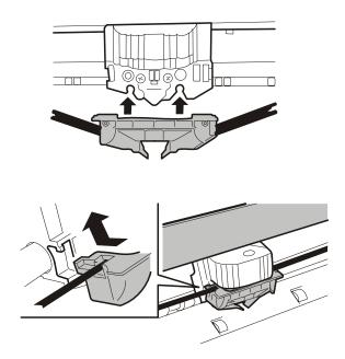
Figure 3-12 Attachment of the ribbon guide
