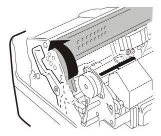
Figure 3-9 Lifting of the upper unit of the mechanism
