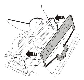
Figure 3-11 Attaching the cartridge to the structure
