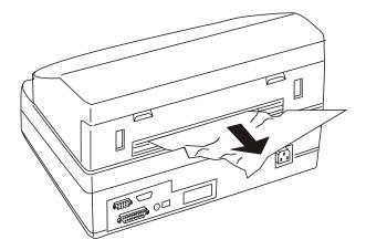
Figure 3 - PR2 plus - Removal of the document in the area of the rear slot
