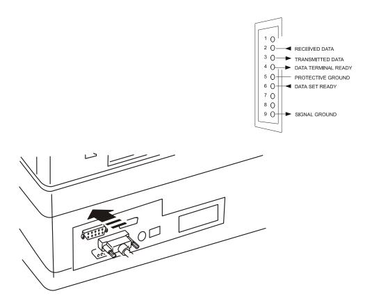
Figure 3-4 Standard RS232C serial interface
