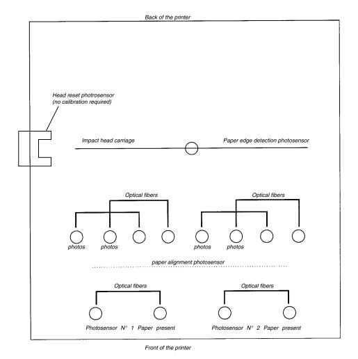
Figure 4-1 Position of machine photosensors
