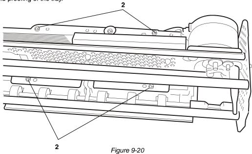
**Note:** During reassembly, check correct positioning of the transmission coupling and of the sound-proofing before tightening the screws.
