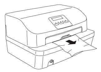
Figure 3-14 Removal of a document in the area of the front feeder
