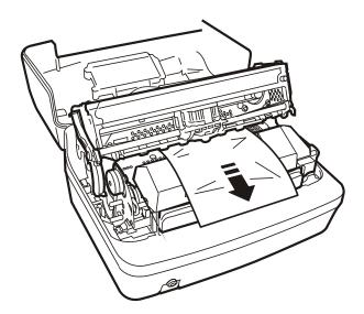
Figure 3-15 Removal of document from inside the printer
