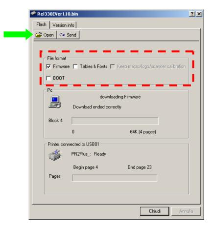
• Select the file containing the firmware to be transferred, confirming this with the Open key.
